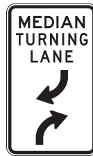
Median turning lane sign
