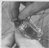
Remove the axle from the hub body. Some hubs may have rubber/metal dust seals covering the inner locking nuts on the outside of the hub body and these can be easily removed with a small screwdriver. Once the seals have been removed, the 13mm cone spanner is used to hold the inner cone section of the axle in place while the 17mm spanner is used to unlock the nut and release the tension between the inner cone and nut before threading the locking nut and cone off the axle completely.
