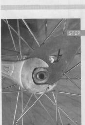
The locking nut and cone need to be locked together firmly and the technique is to make sure that the axle is spinning smoothly without any side-toside movement.
